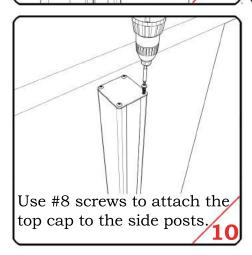
The side post can be mount on: Concrete columns, block wall, house with siding or staccu, fence post or anything stable enough to support the gate's weight (75lb-81lb).
